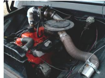
Wood gasification is probably not for everyone. Richard says there is an art to operating the truck, and I can see why. One has to plan when using the wood gasification system. The wood has to be dry. The wood has to be burning at temperature before it makes a useful gas. And then the user has to control the flow of gasoline and wood gas to optimize performance. A series of gauges help to gauge the performance of the system. Sounds like driving my 1984 Mustang GT.
