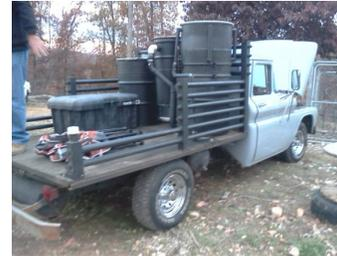
The engine of the truck siphons off the gasified wood as needed with the help of the solenoid and the choke type apparatus located on the engine. The truck is a little underpowered when running on the gasified wood, but even so, it has enough power to function as a normal vehicle. When he needs more power, he just flips a switch and changes back to gasoline.
